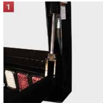
1 Dual hydraulic cylinders ensure a stable and even lift for cargo.
