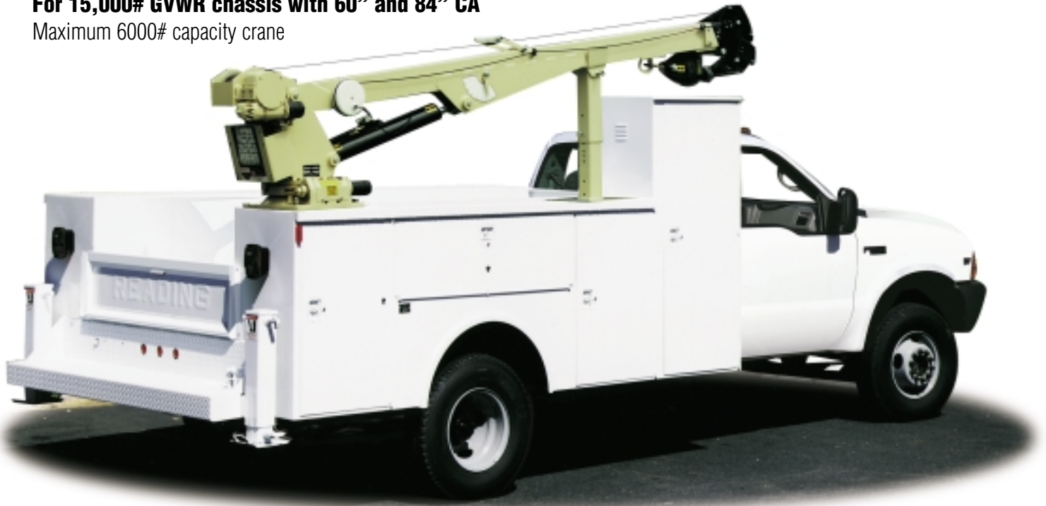
Model shown features standard die-formed fenderettes, and optional manual out / crank down outriggers
