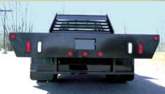
Shown with optional overhead material rack, rear and goose neck tow packages, 4 rear stake pockets, flat tie down rail, and bulkhead lights.
