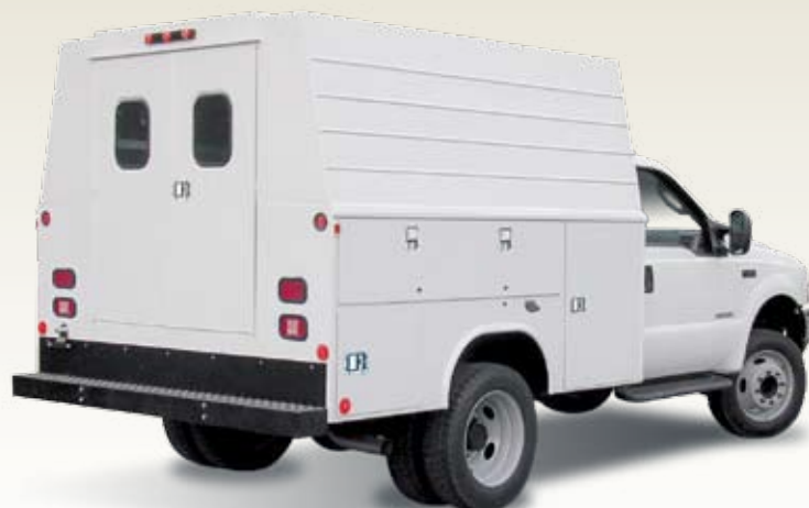
108DW tapered panel body 60 series ("B" side shown) With recessed tail lights and optional pooched anti-slip bumper
