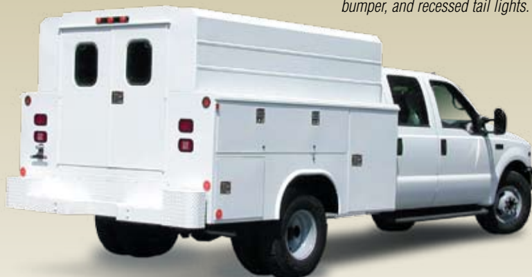
108DW panel body 50 series ("B" side shown) With optional recessed safety step bumper, and recessed tail lights.
